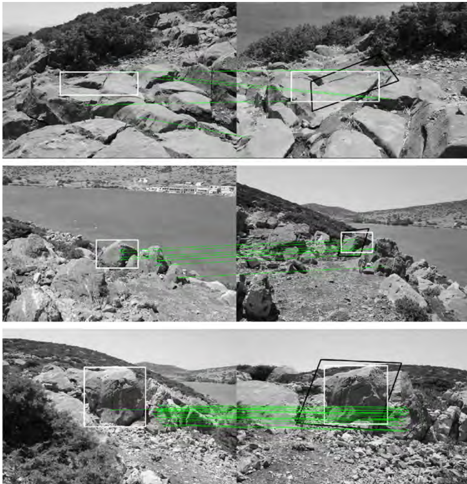
Fig. 4. Detection results using the feature point-based method. An annotated template image is necessary (left column) to perform detection on an input test image (right column). White bounding boxes are manually annotated ground truth rock carving positions. Black quadrilaterals on test images (right column) correspond to the transformed box resulting from the transformation of the ground truth bounding boxes available on the template images (left column). The detected SIFT keypoints that are part of the consensus set are shown, along with the RANSAC-based matches (lines connecting points from one image to the other) between keypoints on each template and test image pair.
